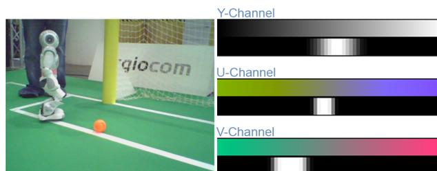
Figure 1: An automatically generated color-table for the carpet based solely on the image on the left.
